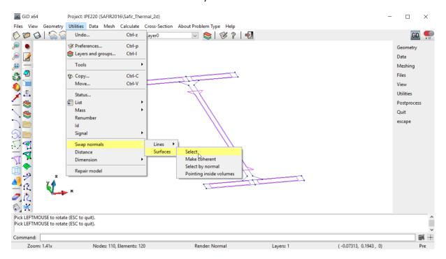
b) For SHELLs, the model will run no matter the way the normals are oriented in the surface entities, but these will define the orientation of the local z axis in the SHELL elements.
