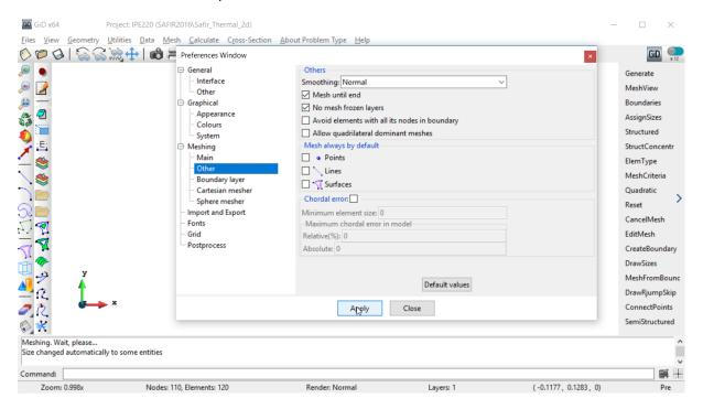
And/or the mesh criteria should be overridden in Mesh > Mesh criteria > No mesh > lines:
