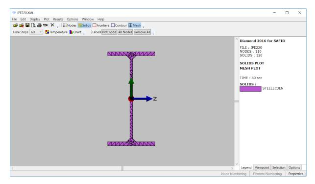
Even if you don't plan to use the cross-section in a structural analysis, the coordinates should be in the surroundings of the origin of the axes, as not doing so may cause problems later in the analysis with SAFIR or in the visualization of results with DIAMOND (i.e., for instance, don't model a section that is built around the coordinates x = 1000m and y = 1000m).
