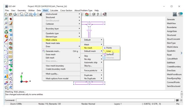
You can check that a correct meshing of the elements has been done after GiD generates the mesh, by looking at the type of the elements meshed in the information box:
