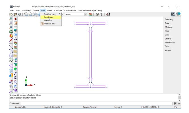
Choose the condition **Torsion Constraint** and apply it to one node in one of the axes of symmetry:
