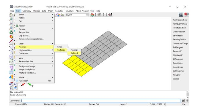
The previous model has different orientations for the surfaces, and hence the resulting SAFIR model will have different orientation of the local axes (image below taken from Diamond).
