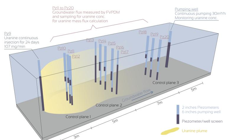
Fig 3: Pz10 to Pz20 are double screen piezometers and are grouped into three control planes. Pz9 is used for Uranine injection (fluorescent dye tracer)
