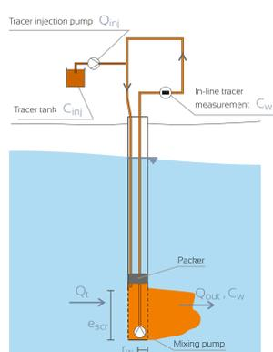
Fig 1: FVPDM experimental setup.
