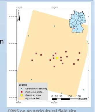
Cosmic Ray Neutron Sensing provides a unique approach to estimate soil moisture dynamics at field scale with high temporal resolution
