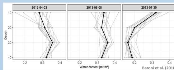
Profiles of a sensor network for days with the same CRNS soil moisture (0.35 m<sup>3</sup> m<sup>-3</sup>). Very different profile shapes and average soil moistures (0.32, 0.34, 0.22 m<sup>3</sup> m<sup>-3</sup>, respectively) lead to the same CRNS soil moisture
