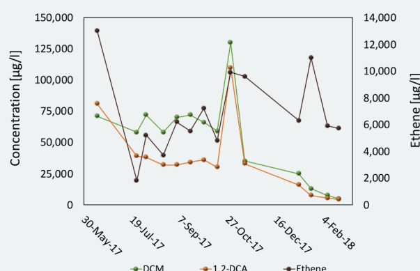
Figure 3. Concentrations of different compounds (1,2 DCA, DCM and ethene) versus time of the central extraction well (EW 15.001).
