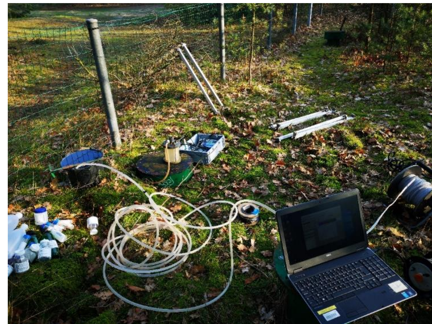
Fig 3. Groundwater sampling setup in the field
