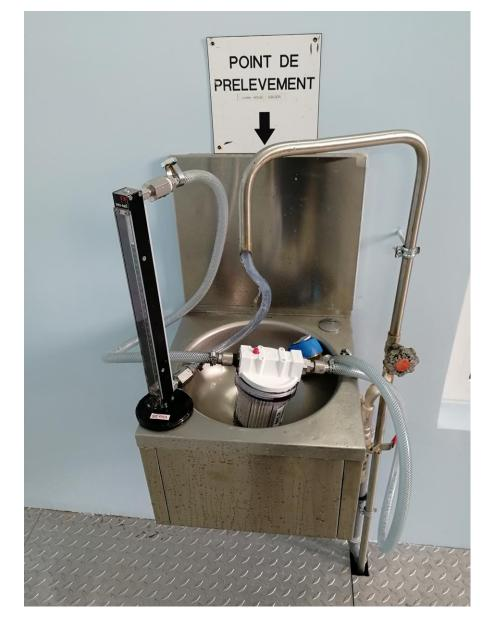
Spring (raw water) Flowmeter Virus sampler Water meter Exit
