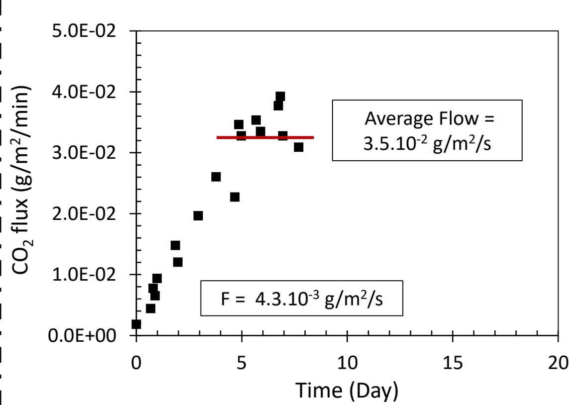
Evolution of CO<sub>2</sub> fluxes until stabilization
