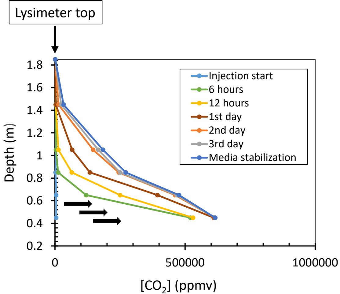
Evolution of CO<sub>2</sub> concentrations at different depth until stabilization
