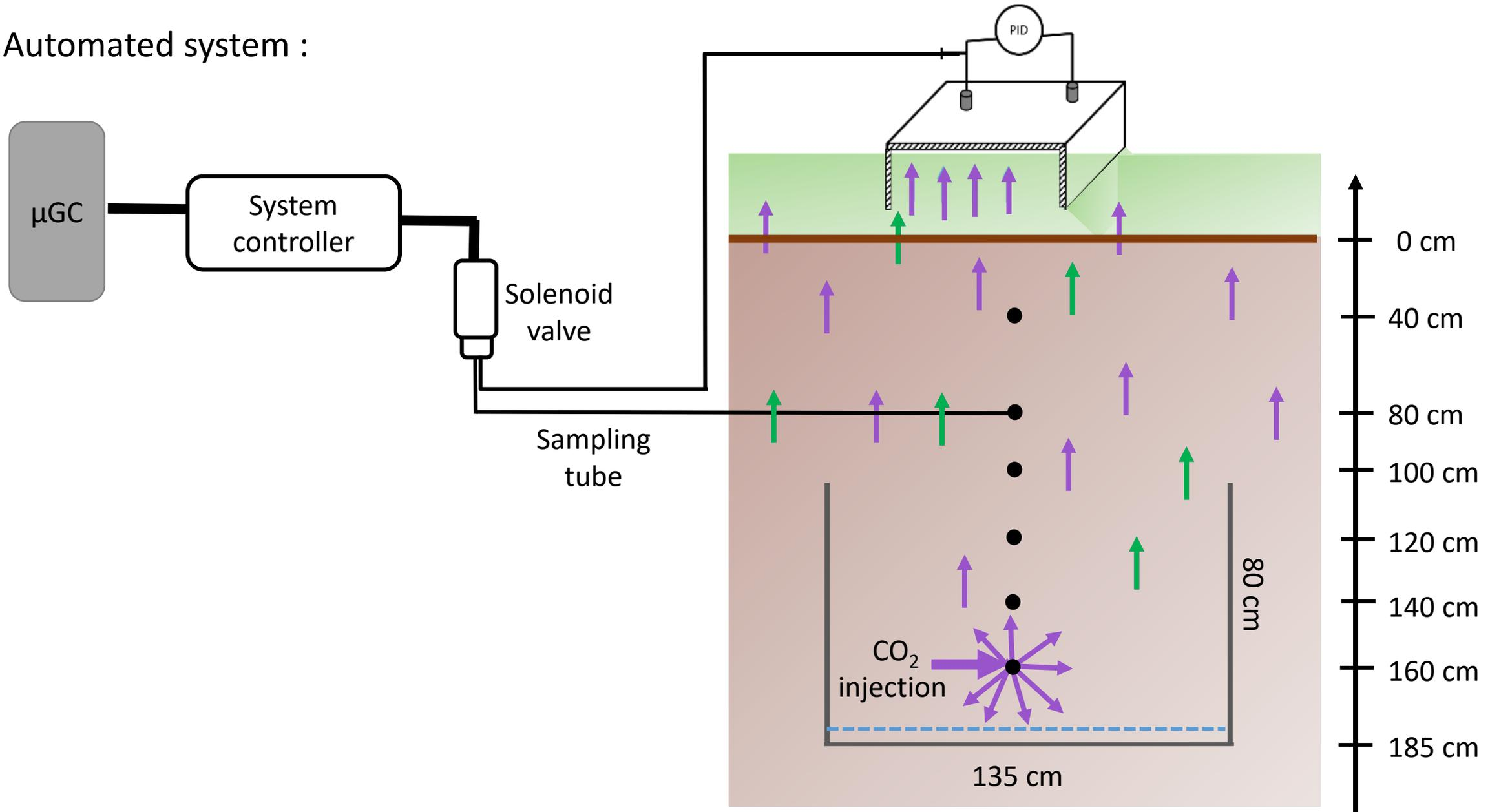
Step 2: A rainfall event was simulated and CO<sub>2</sub> continuous monitoring during a simulated rainfall event
