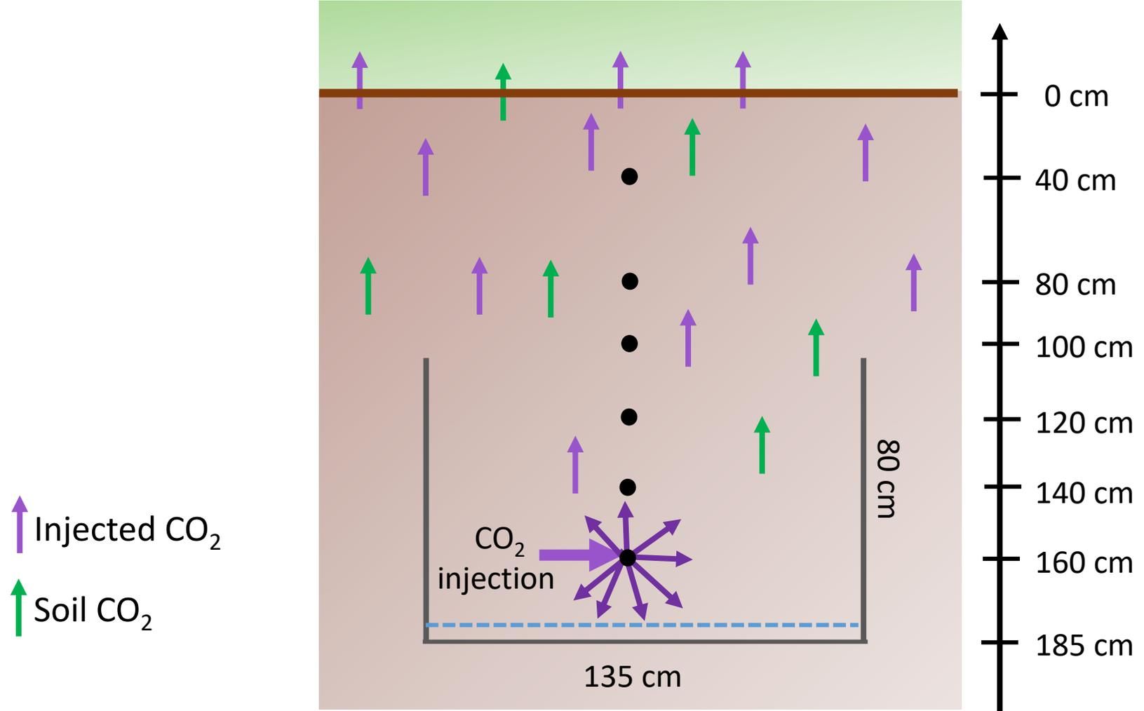
Step 1: CO<sub>2</sub> was injected and gas phase concentration were continuously monitored
