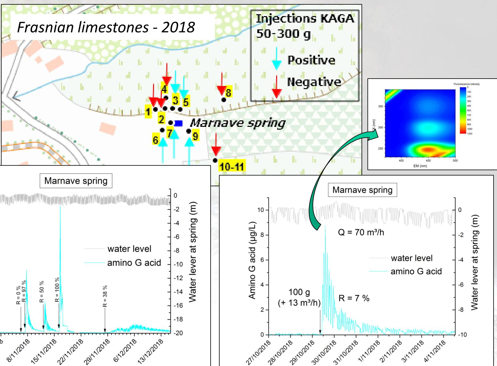
Successive tests with the same tracer (amino G acid) in multiple points
