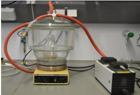
Treatment of the sediment with vacuum and  $N_2$  gas in a desiccator + stirring → **oxygen can be almost completely removed**
