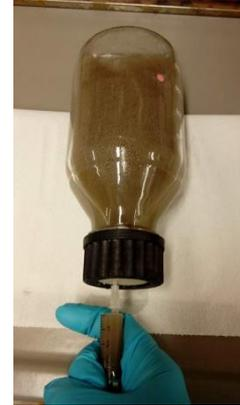
**Denitrifier method:** The technique is based on microbial transformation of nitrate to  $\text{NO}_2$  and the isotopic composition of both nitrogen and oxygen can be investigated
