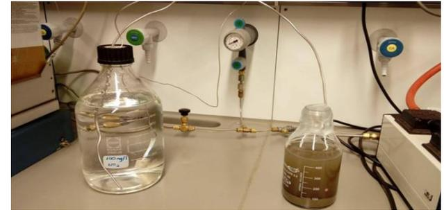
Filling up the soil samples with the solution and sparging with  $N_2$  gas
