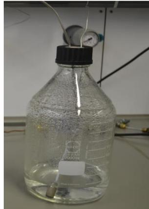
Preparation of oxygen-free, nitrate containing distilled water solution ( $N_2$  gas flushing)
